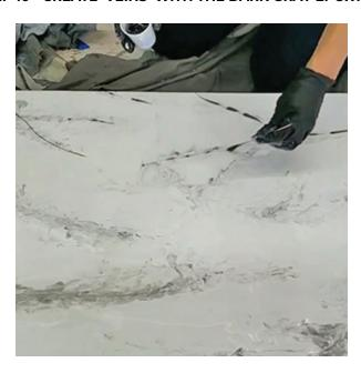
Continue to create the marbling effect by adding dark gray 'veins'. The best place to add veins is on top of, or close to, the light gray feathered areas. Use a clean wooden tongue depressor to apply thin lines of the dark gray mixed epoxy on the surface. Use the heat gun to manipulate the veins.
