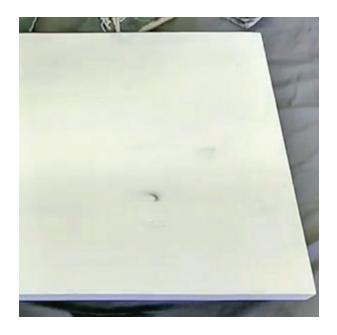
Pour a thin 1/16" seal coat of white mixed epoxy onto the surface, and spread evenly. Wait for the epoxy seal coat to set up and be tack-free before applying your flood coat. If you wait until the surface hardens completely, sand with 220-grit sandpaper, remove residue by wiping with acetone, and let dry.
