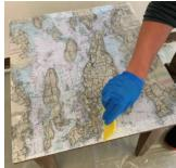
Apply a thin coat of mixed epoxy to seal the surface. After pouring the epoxy, spread it with an epoxy spreader or use the heat gun (keep the heat 6" off the surface, and keep it moving). The seal coat creates an ideal surface for the flood coat to bond to. If you are applying the seal coat to bare wood (instead of a chart, as shown here), the seal coat prevents air in the wood from off-gassing & creating bubbles during the flood coat stage.
