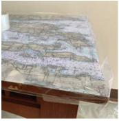
Apply clear packing tape around the edges of the table, to form a dam. Be sure you have at least 1" of tape sticking up beyond the top edge of the table to contain the flood coat(s) of epoxy.
