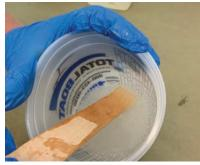
Mix a small batch of TotalBoat TableTop Epoxy for a thin seal coat. Combine **1 part Resin and 1 part Hardener**, by volume.
