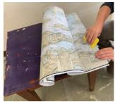
In this example, we're applying an adhesive-backed, plastic-coated nautical chart to the table top. If you are using photographs or other paper items, laminate them first, or use an alternative sealant to prevent damage. It's important to adhere the item securely to the table top before you flood the surface with mixed epoxy.
