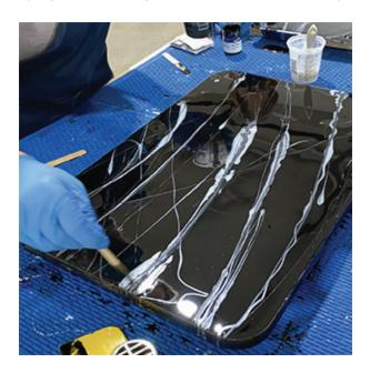
Use a small, clean mixing stick to apply thin lines of the light or dark gray epoxy on top of the silver feathered areas to appear as darker veins in the marble.
